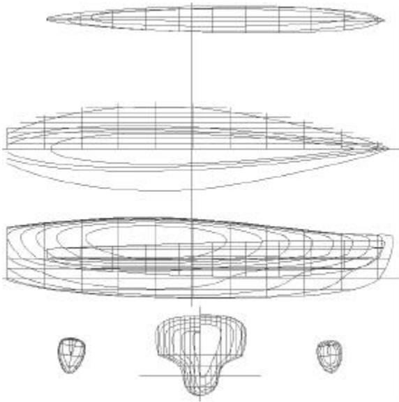
**Fig. 4, Hull Lines**
