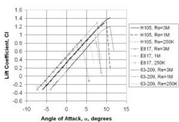
Fig. 19, Section Lift Curves
