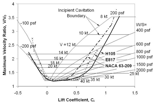
Fig. 21, Maximum Section Velocity
