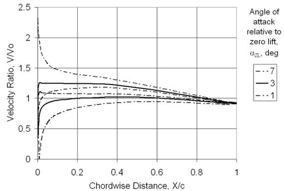
Fig. 16, NACA 63-209 Velocity Distribution
