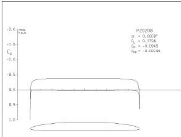
**Fig. 5, P20208 Design Pressure Distribution**
