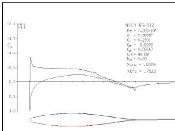
**Fig. 1, NACA 65-012 at 2 Degrees Angle of Attack**
