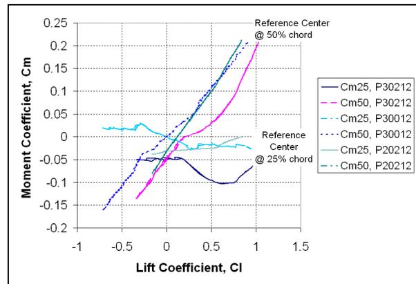
Fig. 26, Moment Coefficient vs. Lift Coefficient
