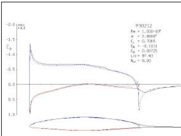
**Fig. 20, P30212 Pressure Distribution,  $\alpha=2.8$  deg.**
