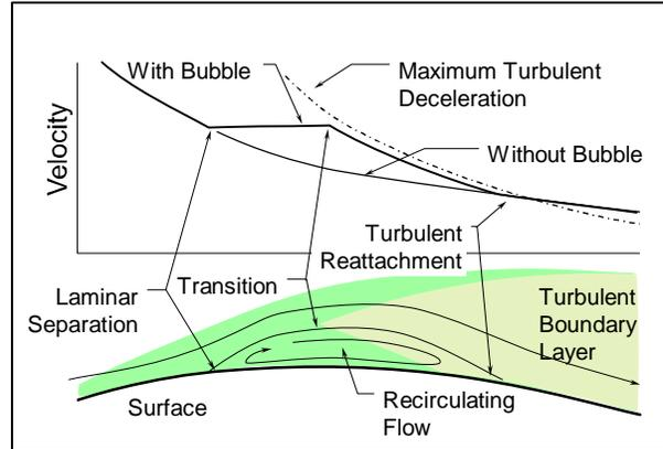
**Fig. 2, Laminar Separation Bubble**
