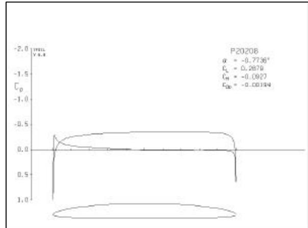
**Fig. 7, P20208 Pressure Distribution,  $C_l=0.29$**
