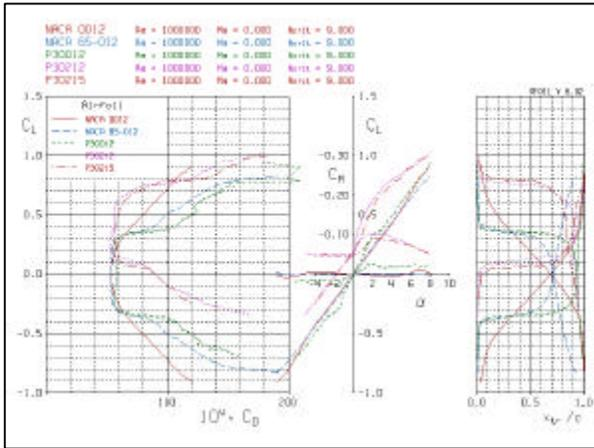
Fig. 23, Proa 3-Series Section Comparison
