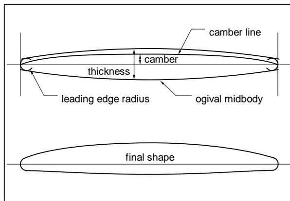
Fig. 2, Proa 1-Series Construction
