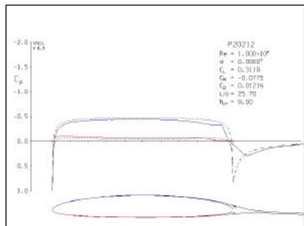
**Fig. 8, P20212 Design Pressure Distribution**
