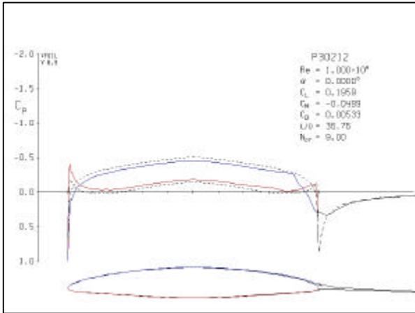
**Fig. 19, P30212 Design Pressure Distribution**
