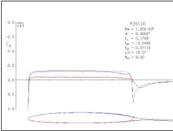
**Fig. 9, P20110 Design Pressure Distribution**
